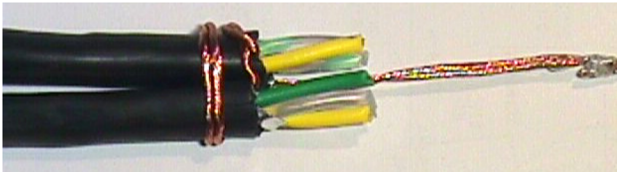
Figure 3 – Bottom view of left side of splice with cable drop
