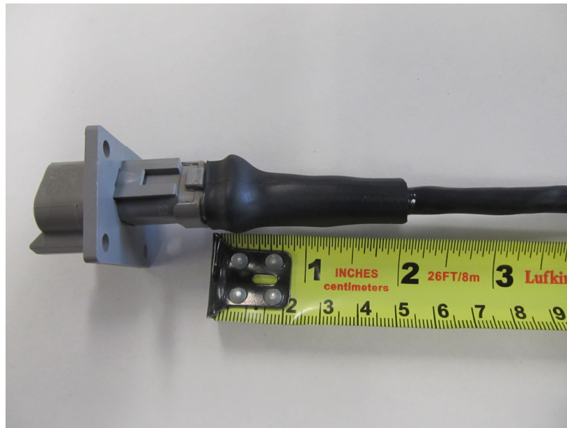
Figure 25 – Finished 3-way connector assembly
