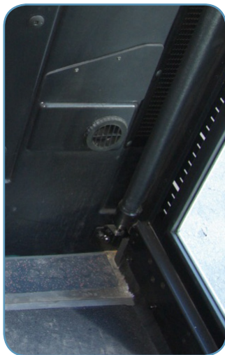
Lower Entrance Door Louver
