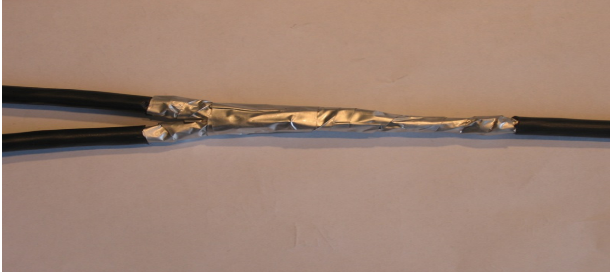
Figure 13 – Cabel after being wrapped with foil wrap
