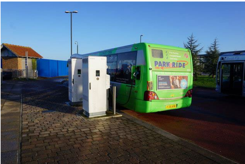
Figure 22. Curbside Charger with Electric Bus
