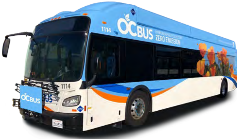
Figure 23. Orange County Transportation Authority Hydrogen Fuel Cell Bus
