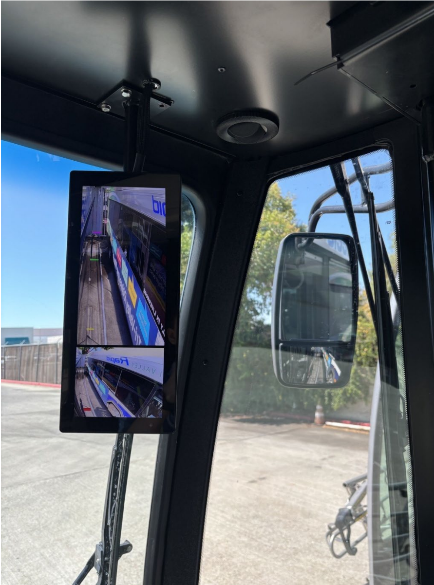
Picture 1: The mirrorless system shown side-by-side next to the traditional rearview mirror.
