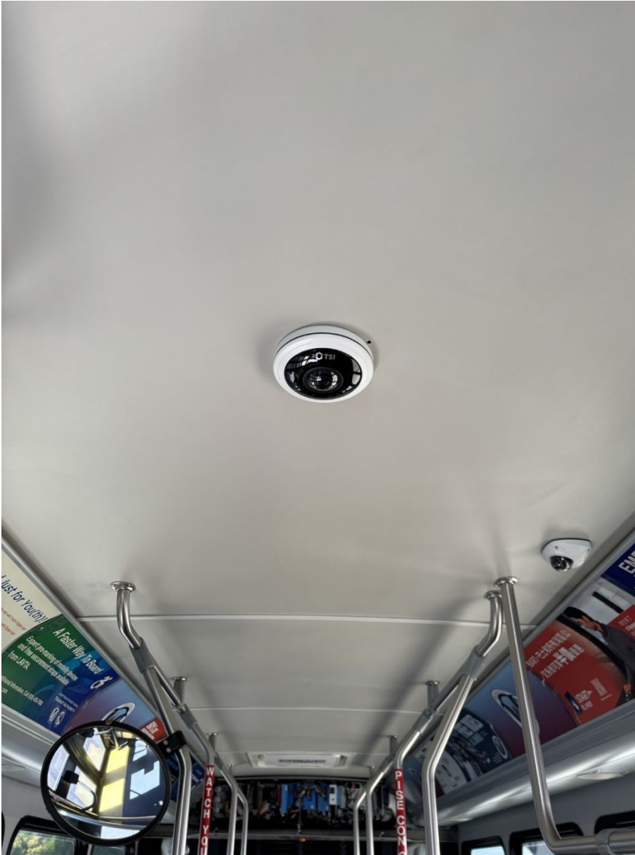
Picture 2: TSL's 360° camera is comprised of multiple cameras contained in one unit, which allows video to be viewed without the "fisheye" effect.
