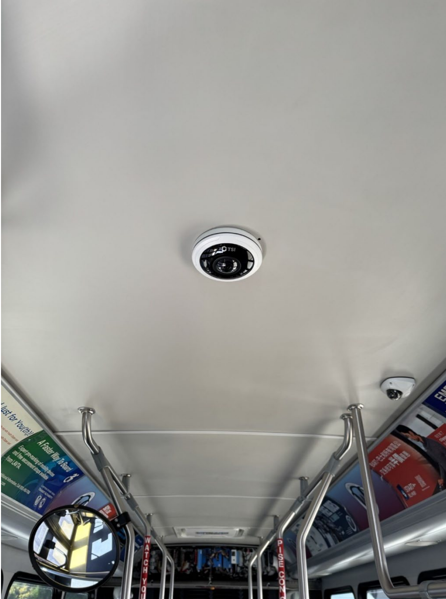
Picture 2: TSI's 360° camera is comprised of multiple cameras contained in one unit, which allows video to be viewed without the "fisheye" effect.
